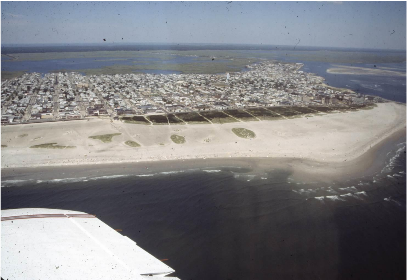
Figure 3. A September 1987 view of the northern oceanfront beach in No. Wildwood showing the original dunes, the massively wide beach complete with 7 dune islands seaward where beach raking debris generated large plant zones on the beach. Note the huge island shoal in Hereford Inlet dividing the inlet into two diverse channels, the one next to North Wildwood hard against the City development with no existing sand beach seaward of the rock revetment at that time. All inlet ebb-tidal sand transport was being deposited on the extensive lobe pushing seaward at 8 th and 9 th Avenues by another 300 feet. The 15 th Avenue lifeguard building is located at the southern end of the oceanfront vegetated dunes and little vegetation if any was present seaward of the boardwalk.
